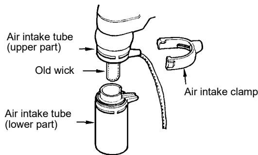
2. Clean the dust on the sensing part (at 30 mm from the top of PT sensor) with alcohol or like. If the old wick is on, remove it. If the new wick is put on the unclean sensing part, the wet bulb indicates temperature higher than actual value.
