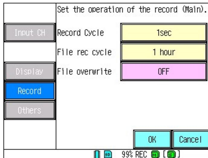
[Record Cycle]: Set the recording interval for main recording.
