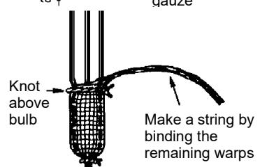
8. Put back the lower part of air intake tube, clamp, and insert the string into the water reservoir. Follow steps 4, 5, 6 in "Replacing the wick".
