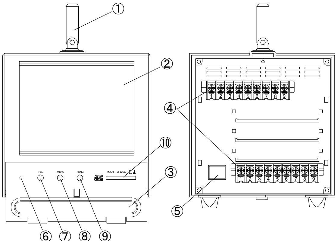
① Handle : Used to carry the recorder by hand
