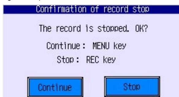
After the recording has stopped, the SD memory card communicates with this equipment to store the data. Do not remove the SD memory card until the data has been completely saved. The memory status indicators will remain red while data is being saved, and will turn light blue when data has been completely saved.
