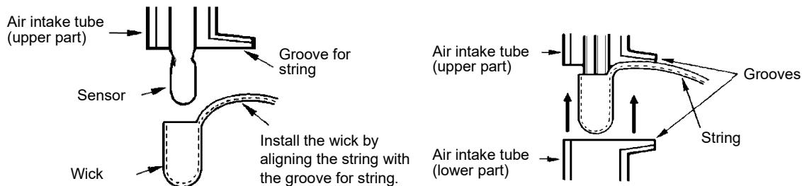
4. Let the string align along with the groove for string and join the upper and lower sections of the air intake tube. At that time, don't let the string get stuck or caught between the housing and air intake tube, between the clamp and air intake tube or in the grooves.
