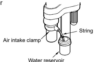
2. Fill the water reservoir to four-fifths with distilled water, using the water bottle supplied (Approx. 13 cc).
