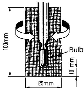
4. Use cotton thread to tie the gauze firmly around the sensing part.
