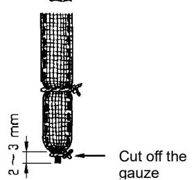
7. Carefully pull out and remove the horizontal threads (woofs) of gauze above the hollow of the sensing part, leaving only the vertical strands (warps). Make a string by binding the remaining wraps of gauze.
