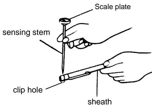
2. Holding the end of the sheath, insert the sensing stem into the target up to the marks (two dents on the stem).
